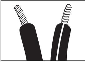
Separate and strip the ends of the speaker wire as shown.
