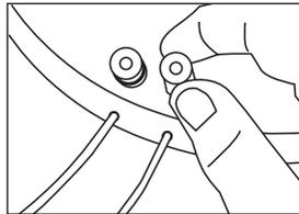
The hole in the center of each collar is intended for use with banana-type connectors. To comply with European CE certification, these holes are blocked with plastic inserts at the point of manufacture. To use banana-type connectors requires the removal of the inserts.
