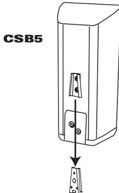
**NOTE:** Remove the base of the CSB5 by removing the two screws on the bottom of the speaker.
