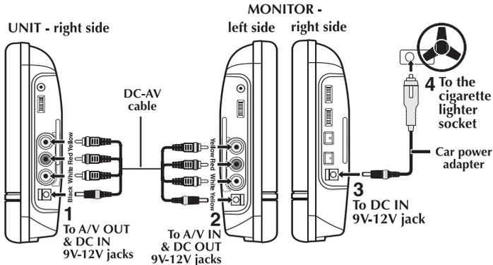
1. Connect the main unit and the monitor using the included DC-AV Cable.
