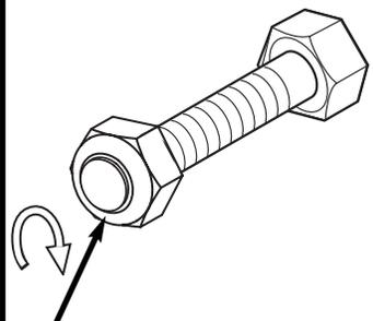
TIGHTEN BOLT (10) IN LOCK NUT (5) UNTIL FLUSH (EVEN) WITH LOCK NUT'S OUTER EDGE.
