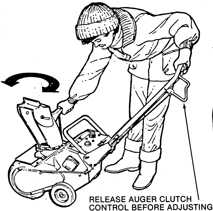
FIG. 8 - STOP BEFORE ADJUSTING CHUTE
