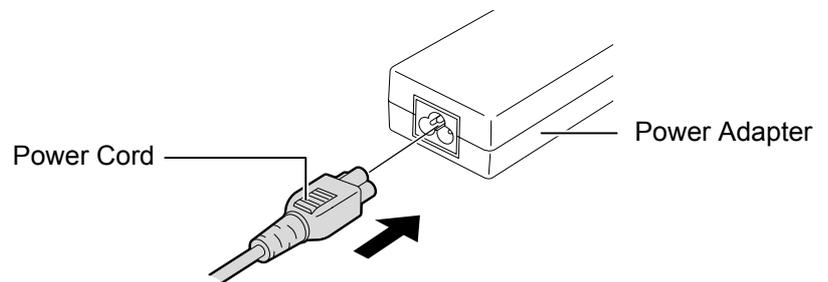
3. Insert the Power Adapter connector into the Power Jack on the rear of the printer.
