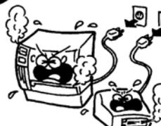
Continued use of the machines in an abnormal condition such as when the machines are producing smoke or strange smells may cause **fire** or **electric shock**. In these cases, immediately turn off the power switches and disconnect the power cord plugs from the outlet. Then, contact your authorised TOSHIBA TEC representative for assistance.
