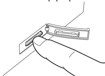
4. Remove it from the slot, and close the SD card slot cover.
