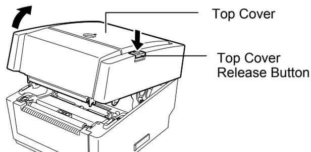
As the Top Cover is held by the damper, it does not close under its own weight.
