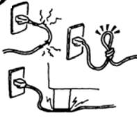
Do not scratch, damage or modify the power cords. Also, do not place heavy objects on, pull on, or excessively bend the cords, as this may cause **fire** or **electrical shock**.
