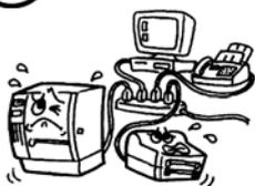
If the machines share the same outlet with any other electrical appliances that consume large amounts of power, the voltage will fluctuate widely each time these appliances operate. Be sure to provide an exclusive outlet for the machine as this may cause **fire** or **electric shock**.
