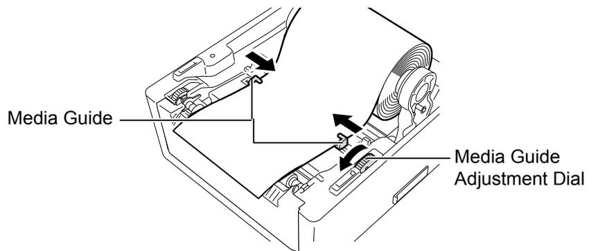
8. Push the Media Holders against the media roll to firmly hold it, then slide the Media Holder Lock Switch to the Lock (▼) side.
