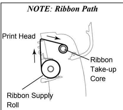
5. Turn the Ribbon Rewind Gear to wind the ribbon leading film onto the Ribbon Take-up Core until the ink ribbon covers the Print Head, and remove any slack of the ribbon.
