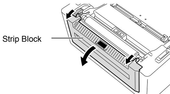
3. Remove enough labels from the leading edge of the media to leave 20 cm of backing paper free, and insert the top edge of the backing paper into the media slot in the Strip Block.
