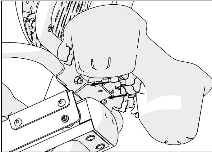
**Figure 11: Bottle holder positioning**
