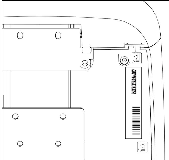
**Figure 16: Serial number label location**
