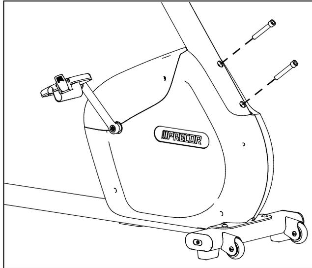
**Figure 14: Bolting the upright support into place**
