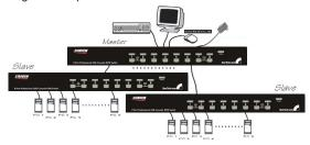
The maximum number of computers controlled in a Master/Slave configuration with all 16-port units is 136, with 8 units of 16-port Slaves (to PC 1 - PC 8) and each Slave connected to 16 computers, plus 8 more computers connected directly to the Master (to ports PC A - PC H):
