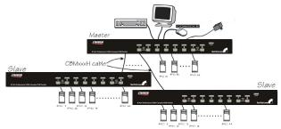
After the connection has been completed, please re-activate the OSD menu to verify that the Master recognizes the Slaves. A triangle mark ( > ) is placed next to the right of the channel name indicating that the port is connected to a Slave, not a computer. A number to the left of the triangle mark indicates the Slave model, i.e. '8' for an 8-port switch.
