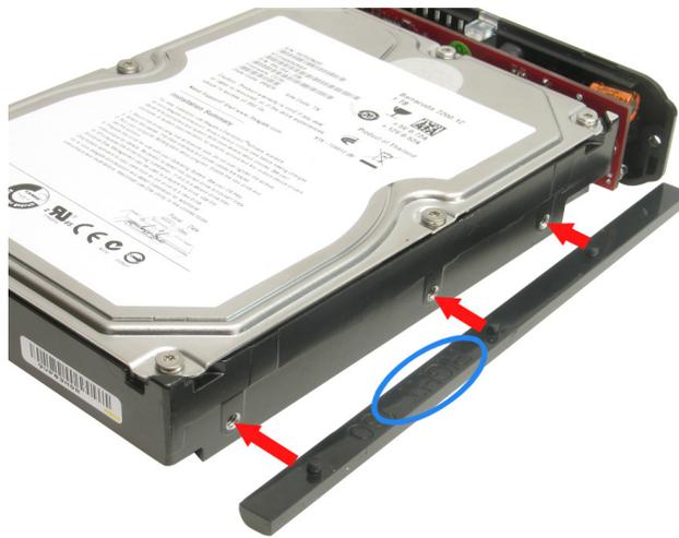
The picture below shows how the guide being attached to the hard drive correctly. If the guides are not properly installed, the hard drive cannot be inserted into the enclosure case.
