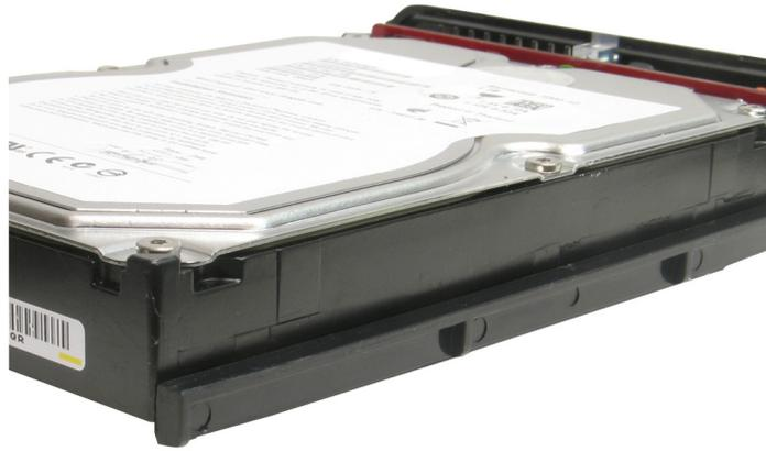
**Step 4** Line up the guides with the case, and slide the hard drive back in. The enclosure should slide shut.
