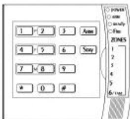
The Orbit-6 can support up to 4 keypads, with a choice of 3 styles, 1 LCD type and two LED types from which virtually all features may be accessed. In addition to the functions it provides for the user, each of the keypads can be used by an installer to program the system parameters.
