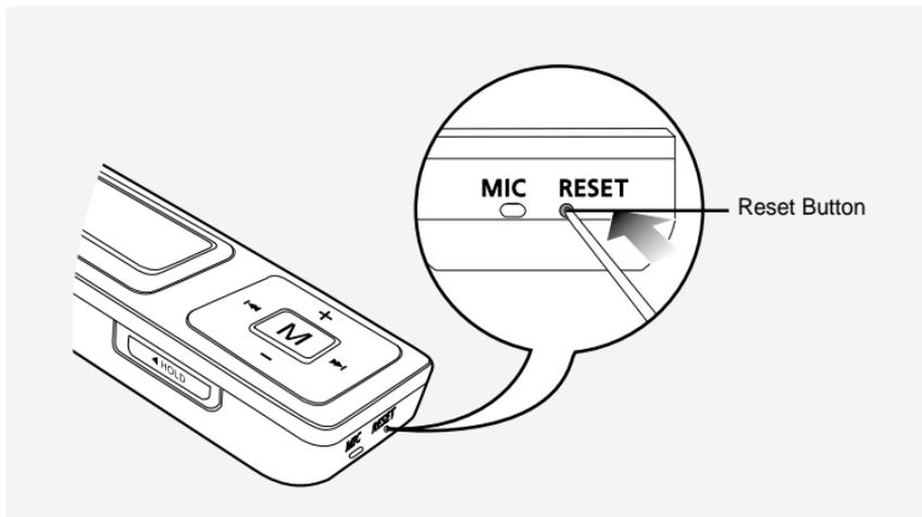
**Press the Reset Button at the bottom of the product with a pointed object such as a safety clip.**
