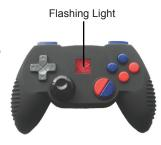
Battery Indicator: A red light will flash when the buttons are pressed indicating the batteries are ok.
