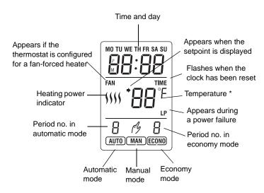
\* The thermostat normally displays the actual (measured) temperature.
