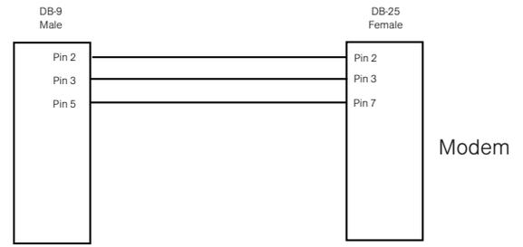
Figure B.3. PSR1212 to Modem RS-232 Connections
