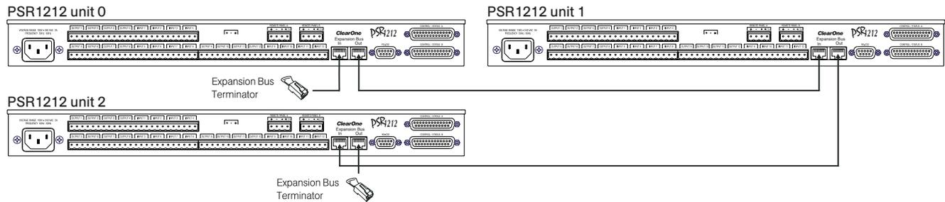
Figure 2.4. E-bus connection diagram
