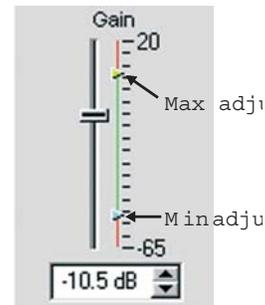
Figure 3.39. Gain adjust on line level input
