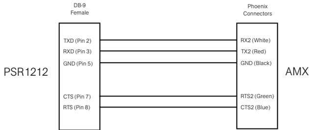
Figure B.4. PSR1212 to AMX RS-232 Connections
