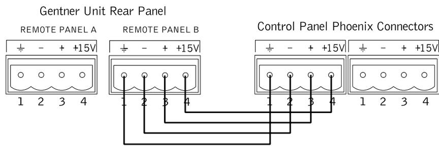
Figure C.3. Wiring the Control Panels
