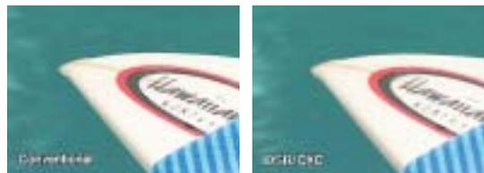
On transition between 2 contrasted zones, the “Black Halo” phenomenon appears. It consists of excess of contrast on the border, the DSP process of the DVCAM camcorders eliminates this phenomenon.
