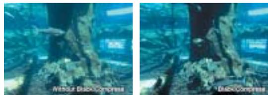
Contrast in the black area of an image can easily be adjusted using the Black Stretch/Compress control function. Black Stretch emphasises contrast in dark areas, while Black Compress enhances or deepens darkness.
