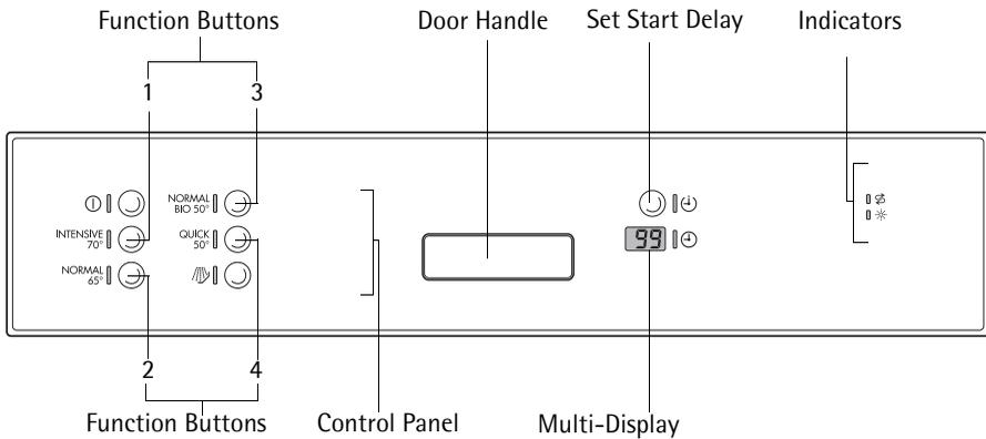
The **control panel** consists of the ON/OFF button
