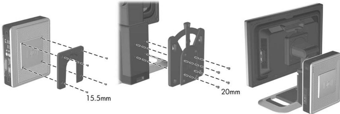
△ **CAUTION:** It is important to verify that the weight of the thin client does not affect the stability of the monitor.
