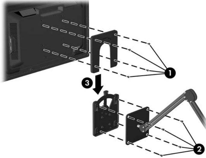
**Figure 3-16** Mounting the Monitor to the Wall Using Quick Release
