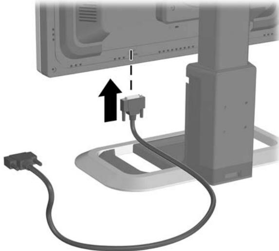
**Figure 3-4** Connecting the VGA Signal Cable
