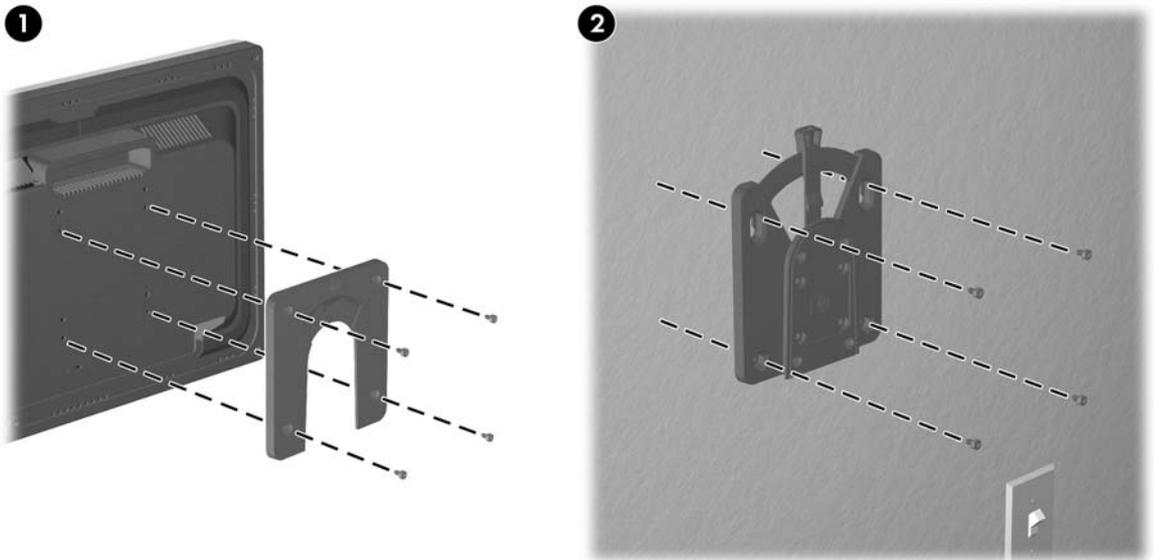
△ **CAUTION:** The Quick Release is designed to support a maximum of up to 24 lbs. (10.9 kg). If you are mounting to a wall, HP recommends that you consult with a qualified engineering, architectural, or construction professional to determine the appropriate type and quantity of mounting fasteners required for the application and to ensure that the mounting solution is properly installed to support applied loads.
