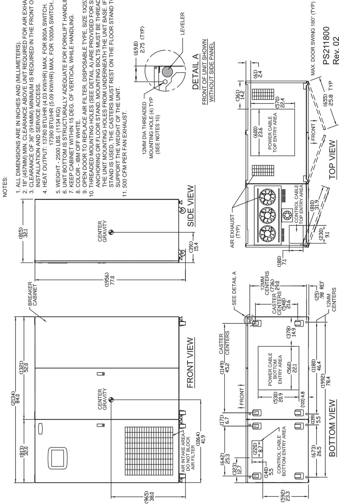
Figure 8 Outline drawing: 100 – 250amp Liebert STS2 with a key lockout switch option
