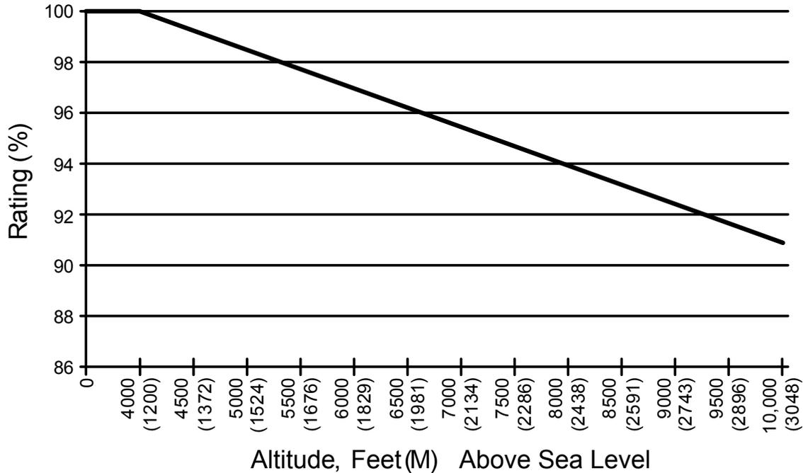
Operation at full load at a higher altitude can be accommodated in ambient temperatures less than 104°F (40°C) ambient. **Figure 2** shows the maximum allowable ambient temperature for full load operation at altitudes above 4000 feet (1200 m).
