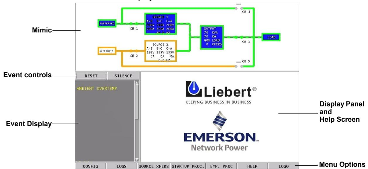
Touch screen control buttons allow you to reset alarms, silence the audible alarm, review configurations, event and history logs, preferred source, startup and bypass procedures, and the help menu. Qualified personnel, with a password, can use these menus to configure parameters, select a preferred source and do manual source transfers.
