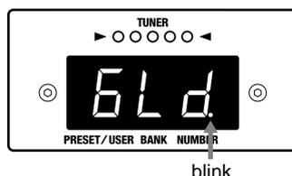
4. When this display disappears, press [SELECT/VALUE ▲] (EXIT) to end the procedure. The user patch you selected in step 1 will be displayed.
