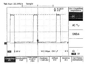
Figure 14B. VCCQP Output Waveform for Output Shorted to Ground
