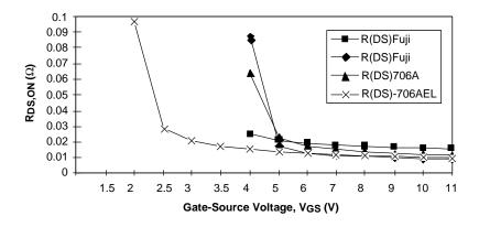
Figure 8. RDS,ON vs. VGS for Selected MOSFETs
