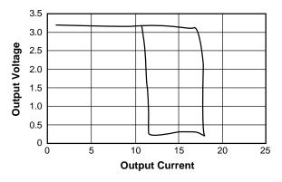
Figure 13. RC5040/RC5042 Short Circuit Characteristic
