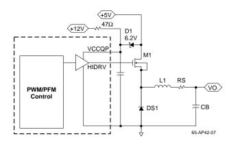
Figure 7. 12V Gate Bias Configuration
