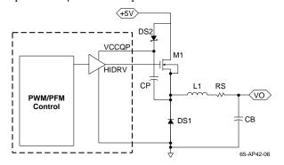
Figure 6. Charge Pump Configuration
