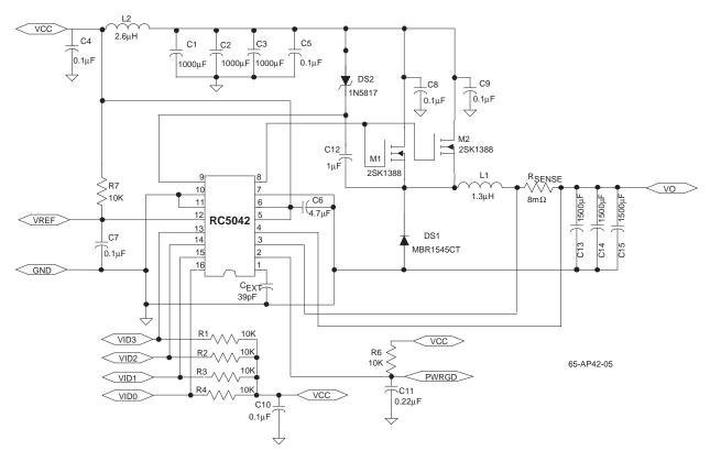
Figure 5. Non-Synchronous DC-DC Converter Application Schematic Using RC5042
