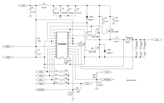
Figure 4. Synchronous DC-DC Converter Application Schematic Using RC5040
