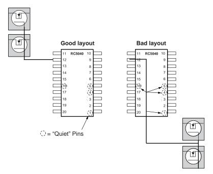
Figure 16. Example of Proper MOSFETs Placements
