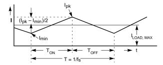
Figure 9. Typical DC-DC Converter Inductor Current Waveform
