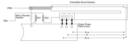
Figure 12. Short Circuit Sense Resistor Design Using PC Trace Resistor and Optional Discrete Sense Resistor
