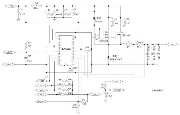
Figure 3. Non-Synchronous DC-DC Converter Application Schematic Using RC5040
