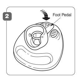
Using your hand or foot, press the foot pedal down to the set position.
