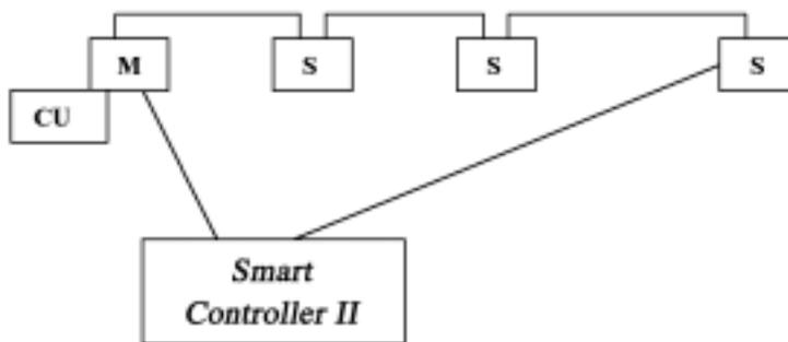
M = Master Evaporator    S = Slave Evaporator    CU = Condensing unit
