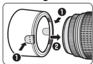
The hood can be reversed and mounted on the lens when not in use.
