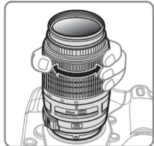
Before focusing, rotate the zoom ring to adjust the focal length and frame the photograph. If the camera offers depth-of-field preview (stop down), depth of field can be previewed in the viewfinder.
