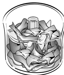
Wrong Water Level for Size of Load
