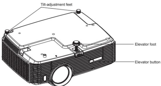
The projector is equipped with an elevator foot to adjust the image height.
