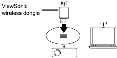
To connect to the projector wirelessly, you have to plug a ViewSonic wireless dongle (optional) to the USB Type A connector on the projector, and then only a few OSD configuration steps are required.
