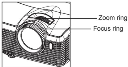
1. Focus the image by rotating the focus ring. A still image is recommended for focusing.
