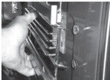
**To remove the oven rack support** for a self-clean cycle, support and lift front bottom of rack support to release front tabs. Then, rotate rack support up and out to release rear tabs. If the rack supports are not removed, the self-clean cycle won't start.
