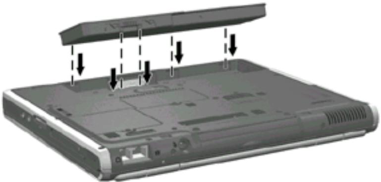
*Inserting the battery pack tabs into the battery bay recesses*
