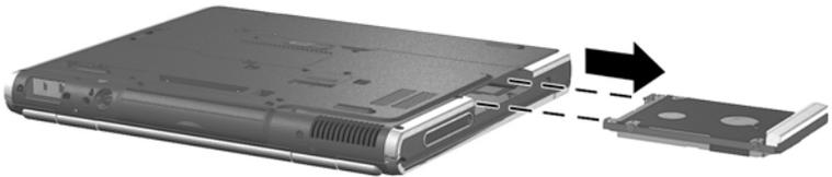
***Removing the hard drive from the hard drive bay***
