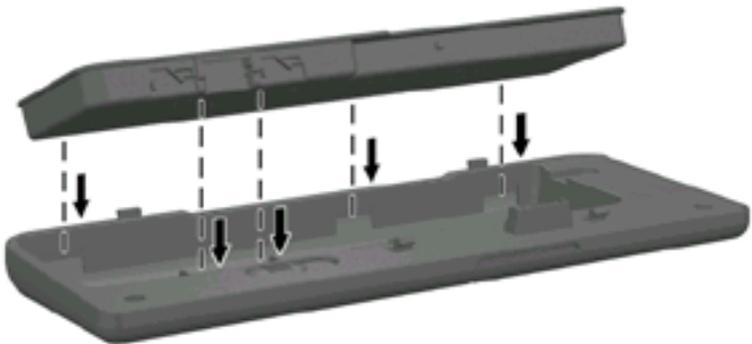
***Inserting the battery pack tabs into the travel battery caddy recesses***
