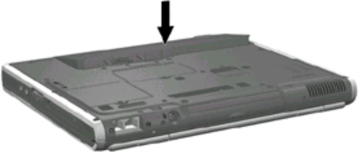
***Inserting the primary battery pack***
