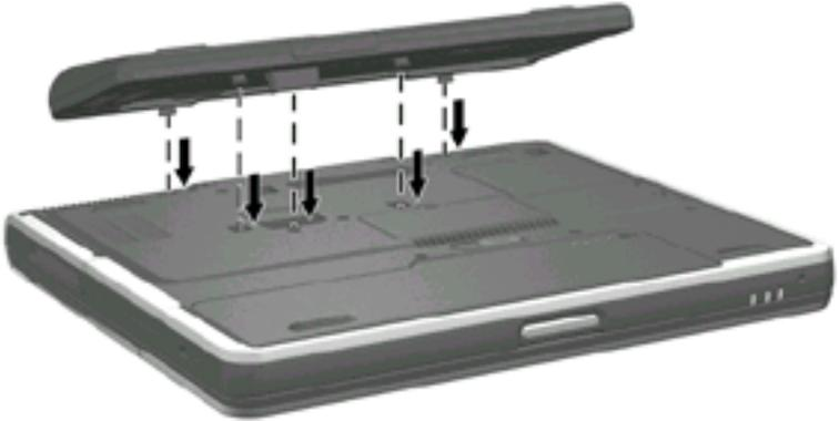
***Inserting the travel battery caddy tabs into the notebook recesses***
