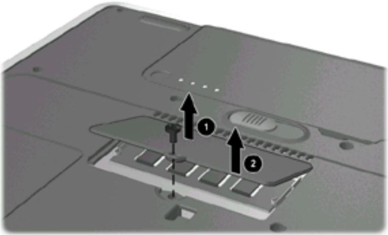
***Removing the expansion slot cover***
