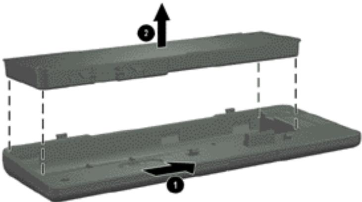
***Removing a battery pack from the travel battery caddy***
