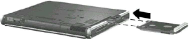
***Inserting the hard drive into the hard drive bay***
