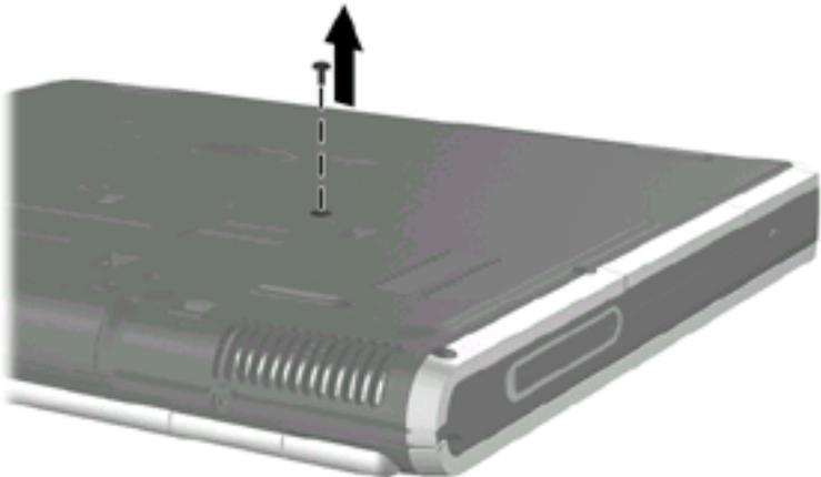
***Removing the hard drive retaining screw***
