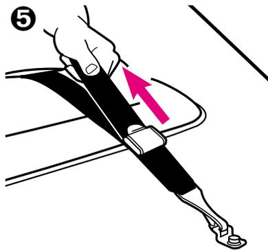
Tighten the tether strap securely. To tighten, pull on free end of strap ⑤.
