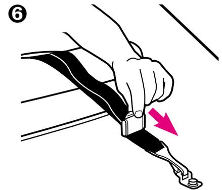
To loosen, lift up on the metal tongue of the buckle ⑥.
