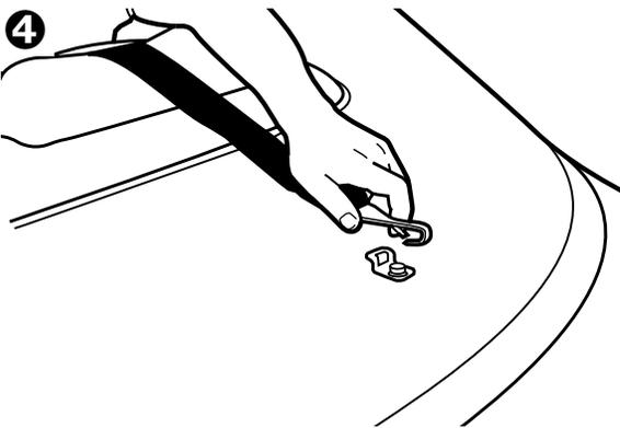
Fasten the tether clip to the anchor point ④.
