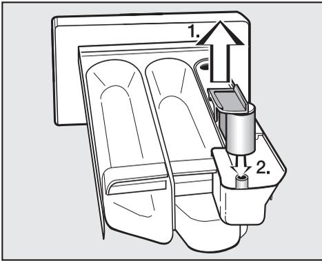
1. Remove the siphon from compartment
