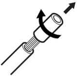
Cut, twist and remove the insulation at the end of each speaker signal cable first, and then, connect the front speakers to the FRONT SPEAKERS terminals by using the cables. You can connect two pairs of front speakers (one pair to the FRONT SPEAKERS ① terminals, and another pair to the FRONT SPEAKERS ② terminals).
