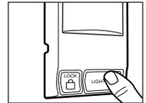
3. Continue holding the ENTER and LIGHT buttons while you press the push bar on the Multi-Function Door Control (all three buttons are held).
