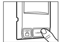
3. Continue holding both buttons while you press the push bar on the Multi-Function Door Control (all three buttons are held).
