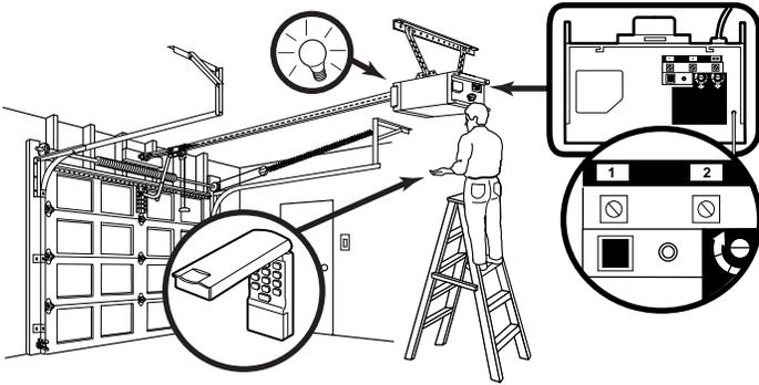
1. Press and release the “learn” button on motor unit. The learn indicator light will glow steadily for 30 seconds.
