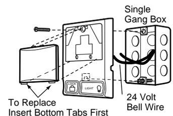
**Figure 3** MULTI-FUNCTION DOOR CONTROL (BACK)
