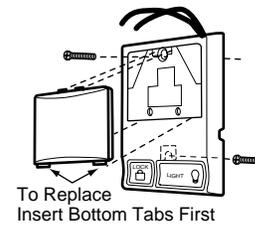
**Figure 2** PRE-WIRED INSTALLATION
