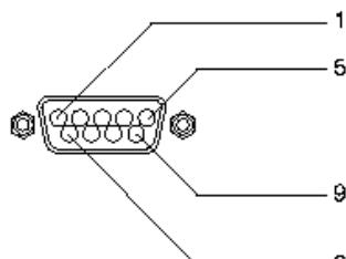
2) Connector on the external equipment side: Serial port (RS-232C) connector. See the specifications of the equipment that is to be connected for the type of connector and the pin assignment.
