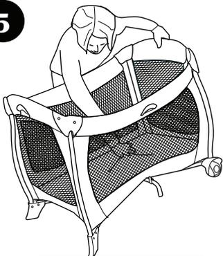
Hold one end of the unit up and push the center of the floor down.
