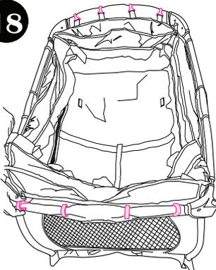
Attach 8 hooks on the bassinet to the ends of the playard as shown.
