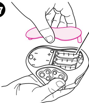
Remove battery door and insert 3 AA (LR6) batteries (not included). Replace door and screws.
