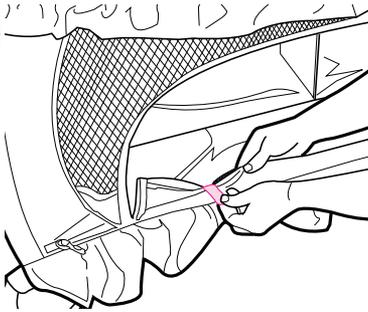
Fasten mesh panel down with hook and loop tabs.
