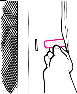
Put two hook and loop tabs under mattress/pad through button holes and fasten securely on bottom of unit.
