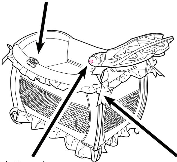
Push button and rotate changing table out of the way when not in use.
