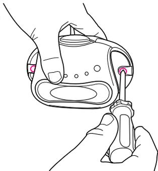
Remove 2 screws from back of electronics module.
