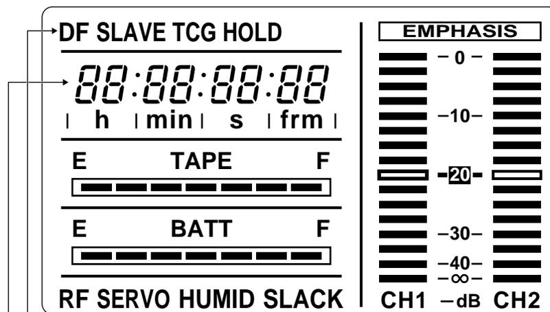
These lamps light to indicate the time code, CTL and real time displays.
