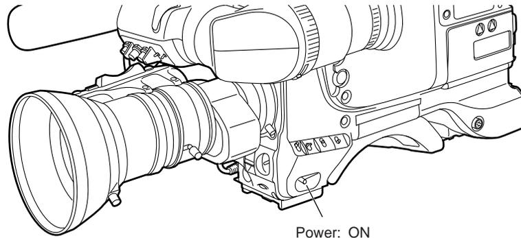
If condensation has occurred inside the unit, the HUMID display lights. In these cases, wait until the display goes off before proceeding to step 2.
