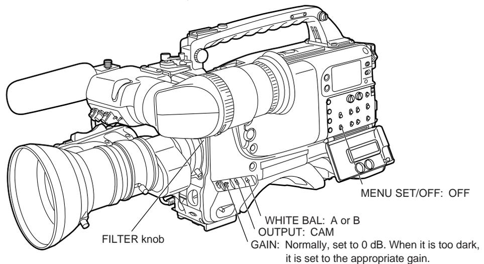
If the settings of the GAIN and WHITE BAL switches are changed, a message informing of the new setting will appear for about 3 seconds at the setting change message display position on the viewfinder screen. (However, the message appears only when the display mode is set to “3”.)
