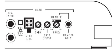
Note: If you are using the Remote Gain, make sure to take this into account during setup procedures of the subwoofer amplifier. You should set the system up with the Remote Gain plugged in and with the level knob turned all the way down (counter-clockwise). The Remote Gain only works when you've selected the LP (low-pass) crossover configuration. On four-channel amplifiers, the Remote Gain only affects the rear channels.
