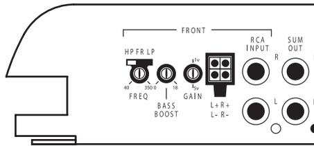
Located on the Input Panel, the objective of input GAIN adjustment is to match the output of the source unit with the input of the amplifier. The output voltage of individual source units can vary. Some source units have an output of 200mV and others have 5 volts or more. To cater to these variations, the amplifier has an adjustable gain level that ranges from 100mV to 5 volts. Follow steps below to set gains.
