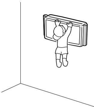
■ **Do not install the Wall Mounting Unit in a location subject to frequent vibration, impact or other external forces.**
