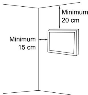
■ **Do not block the ventilation holes, and be sure to leave sufficient space around the unit for ventilation.**
