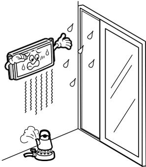
■ **Do not install the Wall Mounting Unit in a location which is hot or humid or which may become wet, as the presence of excessive moisture may lead to fire or electric shock.**
