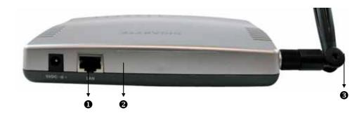
The Wireless LAN Access Point's ports are located on the router's rear panel and the antenna is located on the side panel.
