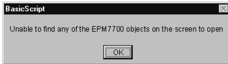
The displayed graphic resulted when an EPM7300 small faceplate was configured to open a screen containing only an EPM 7700 device graphic wizard.
