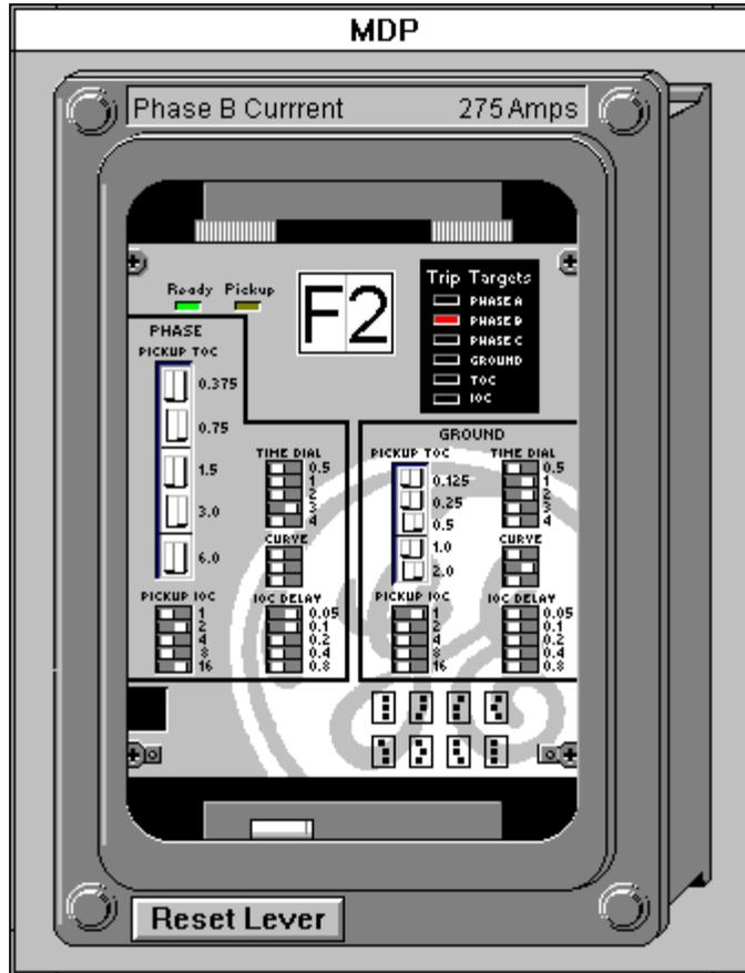
The large faceplate representation of the MDP Digital Overcurrent Relay provides the following animated functions:
