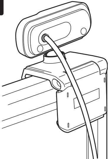
Mount the webcam on your monitor. Unfold the foot and rotate the ball joint as desired.
