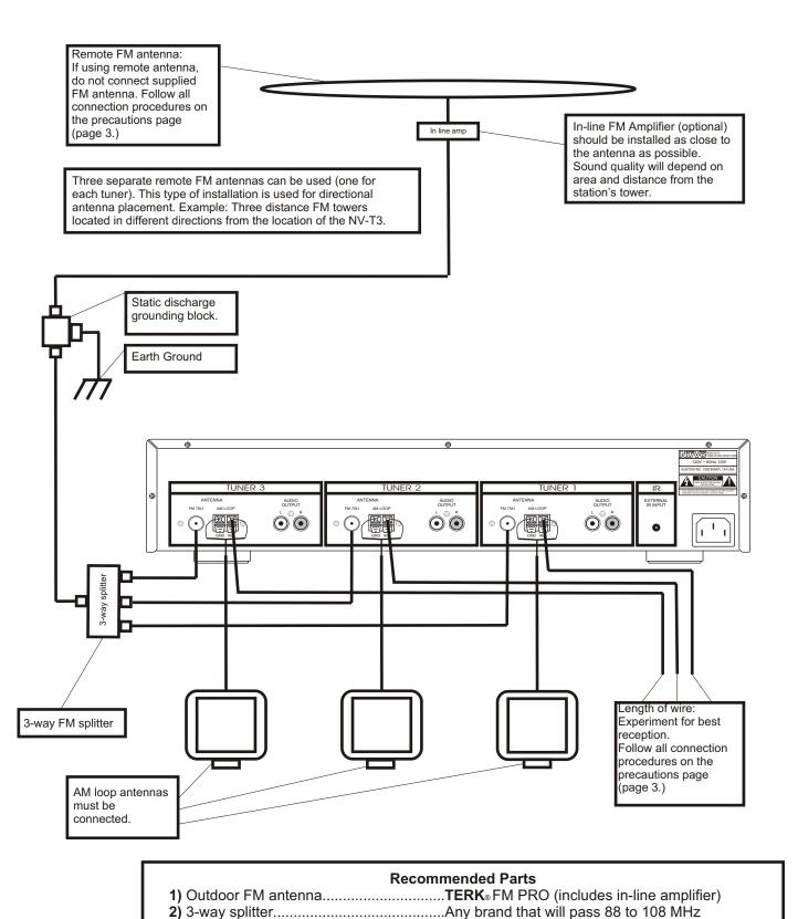
3) Static Discharge Grounding Block......Any brand
