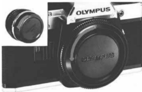
① Remove the body cap and the rear lens cap.\*
