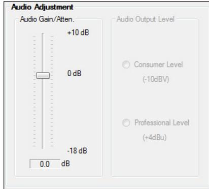
**Audio Gain and Attenuation** — Adjusts the analog input audio gain or attenuation value. This ranges from -18.0 dB to +10.0 dB in 1.0 dB increments.
