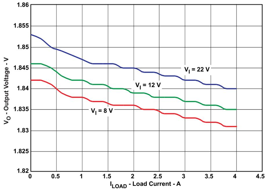
$V_{IN} = 8V - 22V$ ,  $V_{OUT1} = 1.80V$ ,  $I_{OUT} = 0A - 4A$
