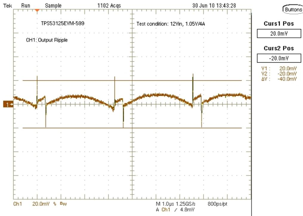
$V_{IN} = 12V$ ,  $V_{OUT1} = 1.05V$ ,  $I_{OUT1} = 4A$
