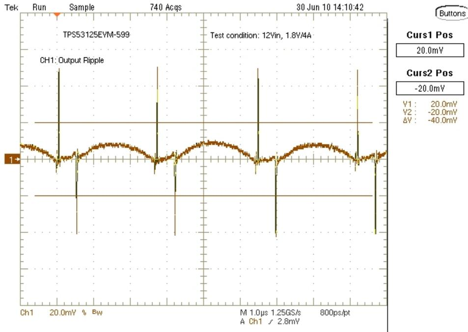
$V_{IN} = 12$ ,  $V_{OUT2} = 1.80$ ,  $I_{OUT2} = 4$  A
