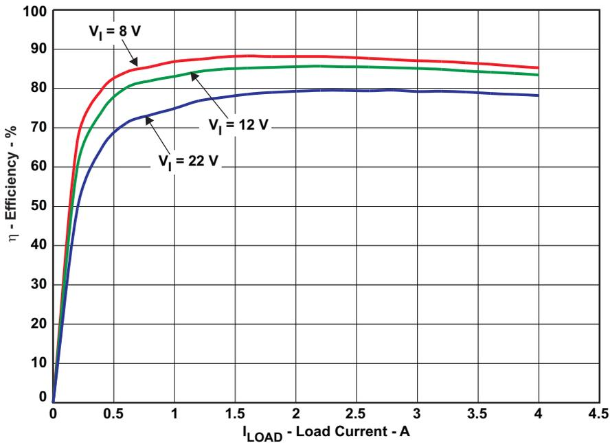
$V_{IN} = 8\text{ V} - 22\text{ V}$ ,  $V_{OUT2} = 1.80\text{ V}$ ,  $I_{OUT2} = 0\text{ A} - 4\text{ A}$
