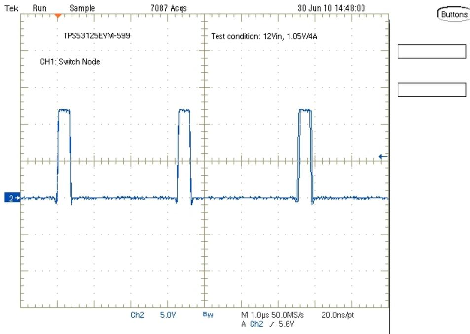
$tV_{IN} = 12$ ,  $V_{OUT1} = 1.05$ ,  $I_{OUT1} = 4$  A,
