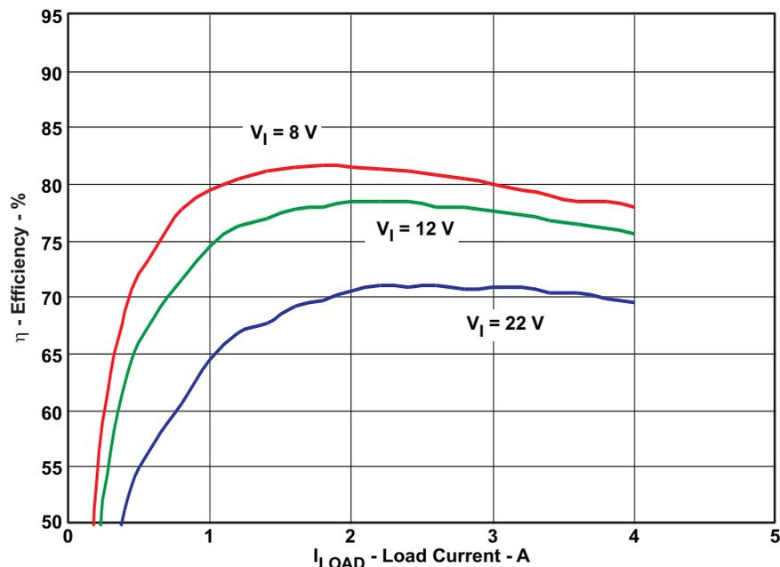
$V_{IN} = 8V - 22V$ ,  $V_{OUT1} = 1.05V$ ,  $I_{OUT1} = 0A - 4A$
