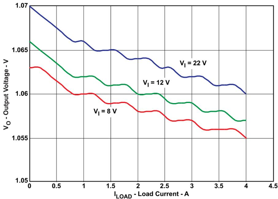
$V_{IN} = 8\text{ V} - 22\text{ V}$ ,  $V_{OUT1} = 1.05\text{ V}$ ,  $I_{OUT} = 0\text{ A} - 4\text{ A}$
