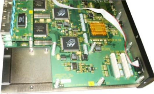
Looking down into the Magnum 6K32T unit, notice that there are individual PM installation spaces and female latch (white) connectors provided on the far right side of main board along with four stand-off's for 6KPM card position. (See Figure 3.5.1c).
