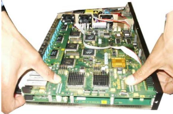
color latching connectors (male) placed at the bottom of the daughter board with the other female connector placed on the Granddaughter and main board. As shown above in Fig. 3.5.2e
