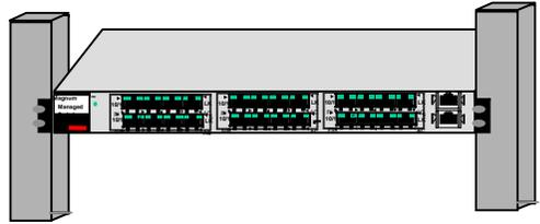
then typically fastened into a standard 19" RETMA rack as shown here
