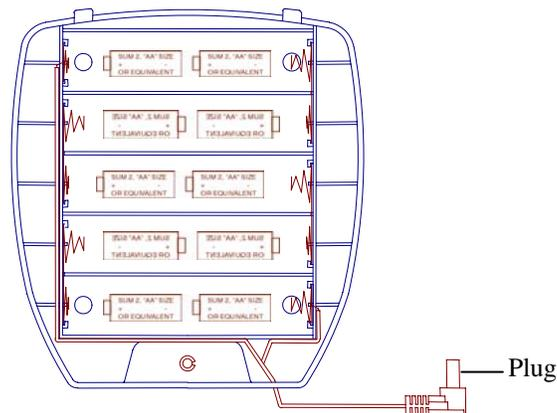
Your wireless monitor has both AC or battery option. When using the AC option with rechargeable batteries, your monitor will automatically switch to back up battery feature during a power outage providing you with uninterrupted power to the monitor. The battery option also provides you the flexibility to move the monitor from room to room. Battery life is approximately 2 –3 hours
