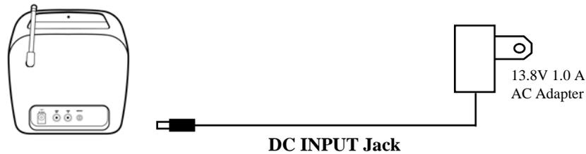
1. Connect the supplied 13.8V AC adapter to the DC INPUT JACK at the rear of the receiver monitor and plug it into an electrical outlet.
