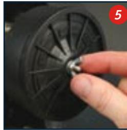
5. Replace the air filter holder, then the air filter, cover and washer and wing nut.
