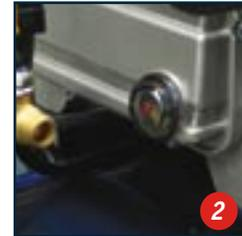
2. Use the oil supplied to fill the crank case until the oil level as seen in the oil level glass (16) is up to the mid point of the red circle.
