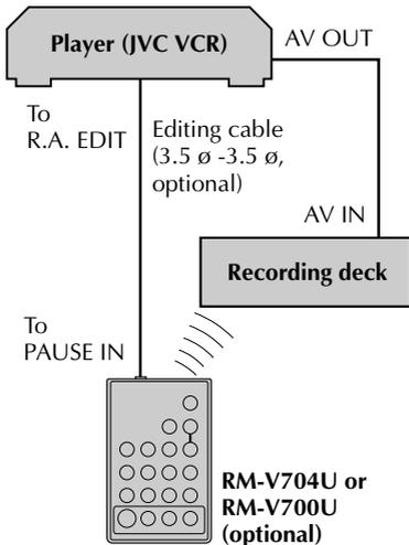
Using the RM-V704U/V700U remote control, it is also possible to perform deck-to-deck Random Assemble Editing. The playback deck must be an R.A. Edit-capable JVC VCR. The recording deck can be...
