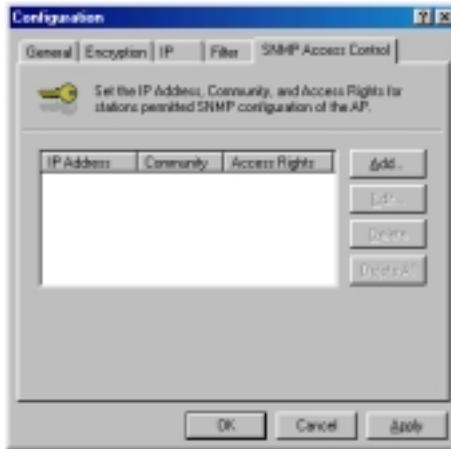
**Figure 14. Configuration/SNMP Access Control**
