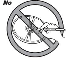
Do not use any solvents such as commercially available cleaners, anti-static spray, or thinner to clean compact discs.
