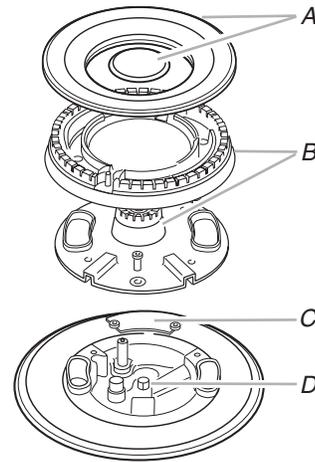
**IMPORTANT:** The TripleTier® Flame burner has 2 gas orifice spuds. Do not forget to change the external gas orifice spud located under the plate.
