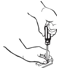
Depending on the thickness of your flooring, longer screws may be necessary to anchor the bracket to the subfloor. Longer screws are available from your local hardware store.
