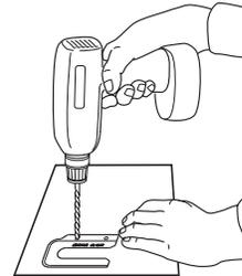
To mount anti-tip bracket to concrete or ceramic floor, use a  $\frac{3}{16}$ " (4.8 mm) masonry drill bit to drill 2 holes at the positions marked on the bracket template. Remove template from floor. Tap plastic anchors into holes with a hammer.
