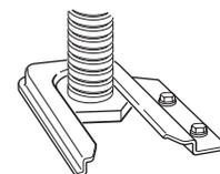
9. If installing the range in a mobile home, you must secure the range to the floor. Any method of securing the range is adequate as long as it conforms to the standards in the "Location Requirements" section.
