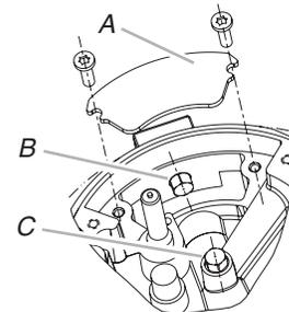
4. Apply masking tape to the end of a 7 mm nut driver to help hold the internal gas orifice spud in the nut driver while changing it. Press nut driver down onto the internal gas orifice spud and remove by turning it counterclockwise and lifting out. Set internal gas orifice spud aside.
