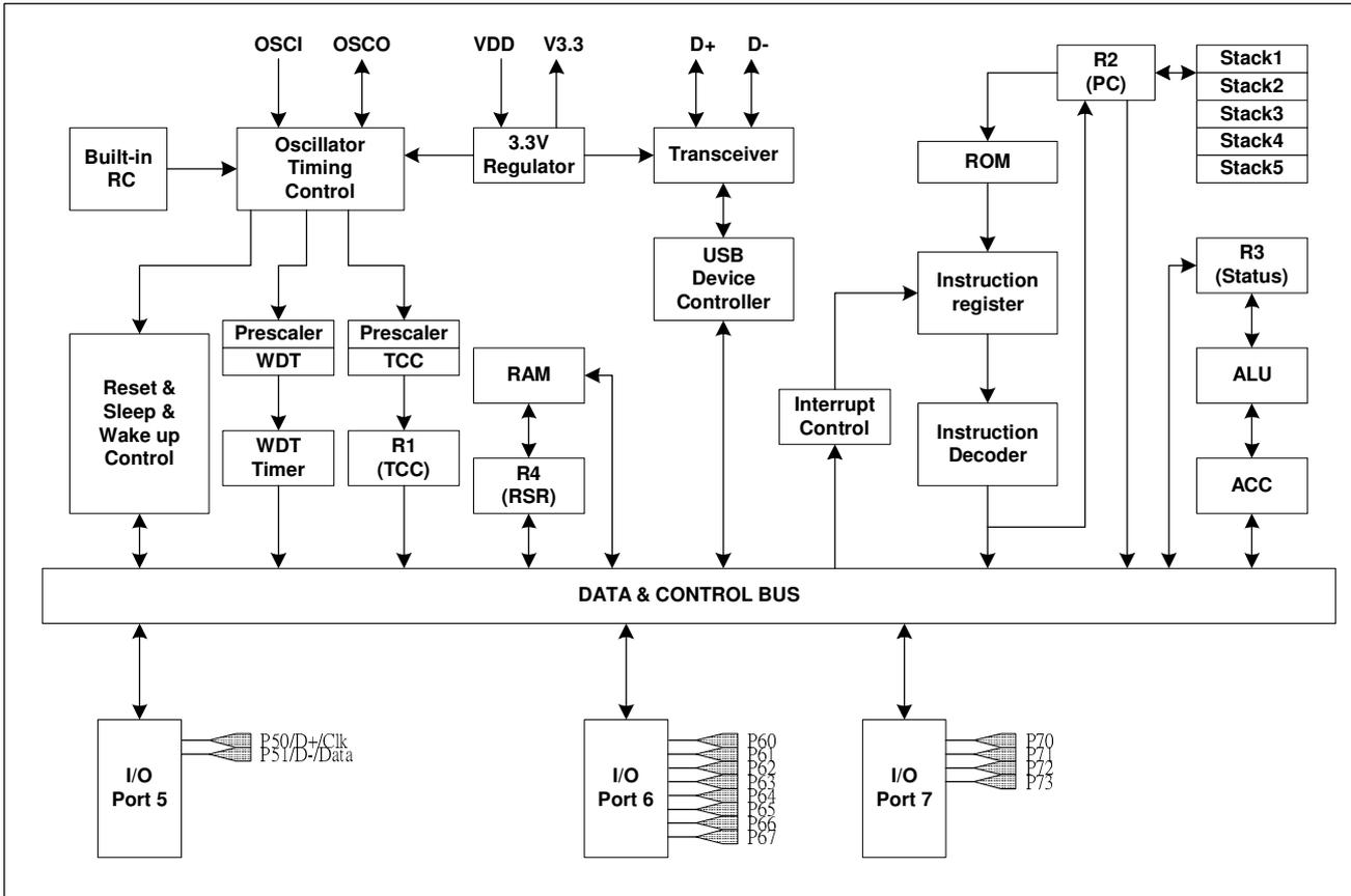
Figure 6-1 EM78612 Series Function Block Diagram
